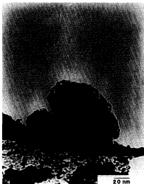
FIG. 14. Micrograph of the same particle as that in Figs. 3 and 7 after oxidation and re-reduction at 673 K. This edge view was taken at a higher magnification than the micrographs in Figs. 3 and 7 to show the irregular structure of the surface. No noticeable change in the overall size of the particle was noted after re-reduction.
