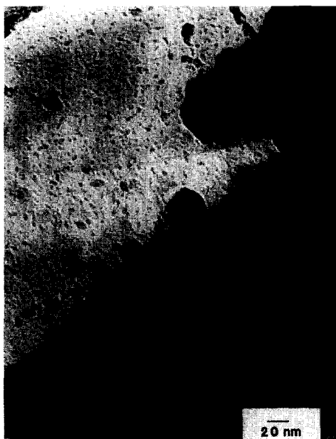
FIG. 10. Micrograph of Mn-only catalyst after oxidation at 523 K and air exposure at 300 K. Note that no void space formed in these particles. The particle sizes did not change as a result of the oxidation pretreatment.
